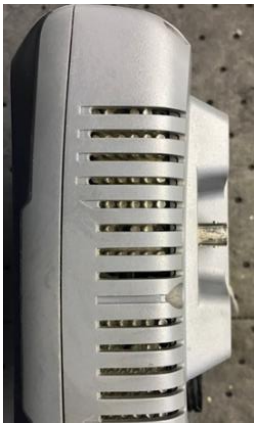
First Generation Non-Repairable Heat Sink can be seen through vent openings
