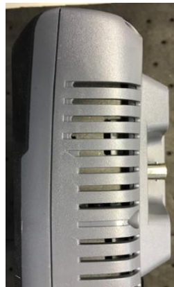
Second Generation Limited Repair Flat metal can be seen through vent openings.
