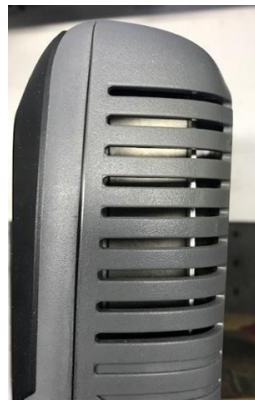
Second Generation Limited Repair Flat metal can be seen through vent openings.
